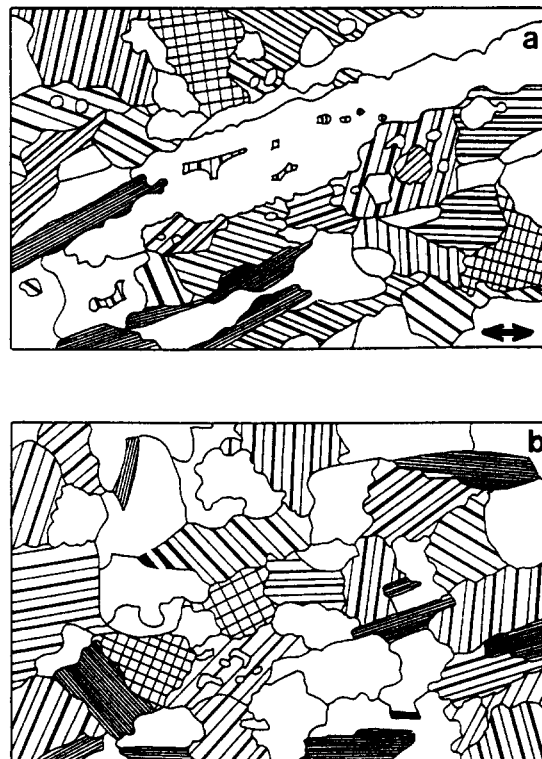
Fig. 7. Line drawing of photomicrograph of ribbon-bearing gneiss. White = quartz; finely hatched = biotite; coarsely hatched = plagioclase; cross hatched = K-feldspar. (a) Section parallel to the XZ -plane of the shape fabric, (b) section parallel to YZ . Note shape fabric of quartz ribbons ( ca 20:3:1), feldspar inclusions in quartz, and lobate quartz–feldspar boundaries. Scale bar 0.5 cm.
